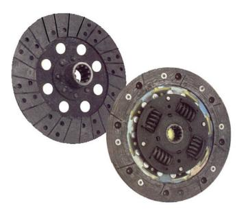
Figure 5.12 Solid and flexible discs
