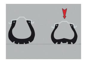
Figure 4.150 Cross-ply tyre profile
