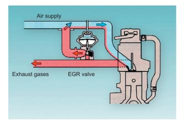
Figure 2.29 Exhaust gas recirculation (EGR)
