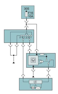
Figure 3.123 Circuit for electric windows
