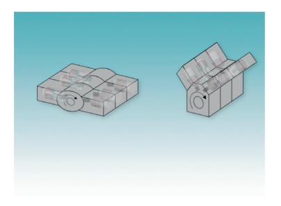
Figure 2.45 Flat and 'V' engines
