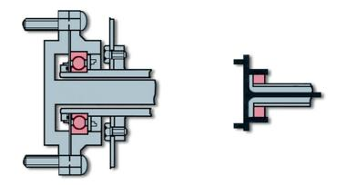
Figure 5.98 Wheel bearing: three-quarter floating
