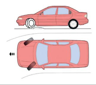
Figure 4.47 Suspension and steering interact
