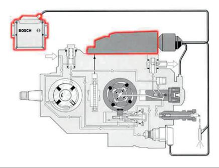
Figure 2.296 Electronic control units
