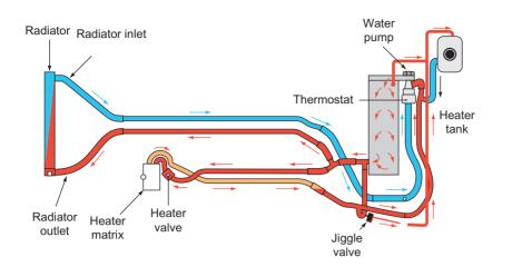
Figure 2.148 Basic cooling system
