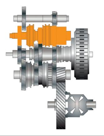
Figure 5.75 Output shaft 2
