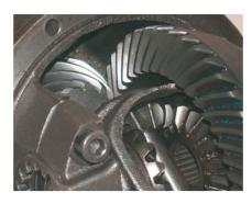
Figure 5.116 This differential is described as an open type
