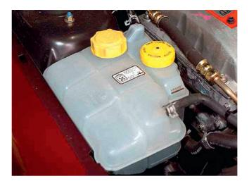
Figure 2.160 Remote expansion tank (on the left)
