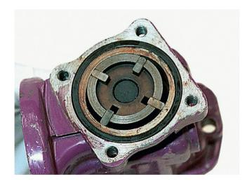
Figure 2.131 Vane pump
