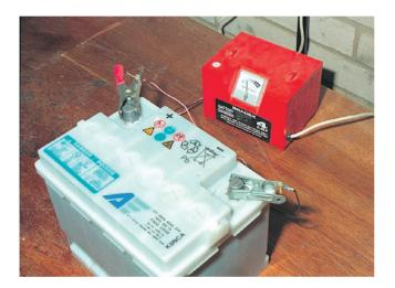
Figure 3.47 Recharging with a small bench charger
