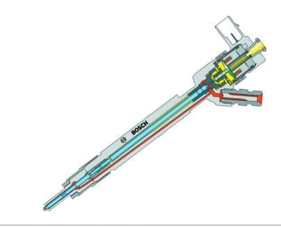
Figure 2.297 Injector. (Source: Bosch Media)
