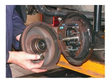
Figure 4.99 Leading and trailing system
