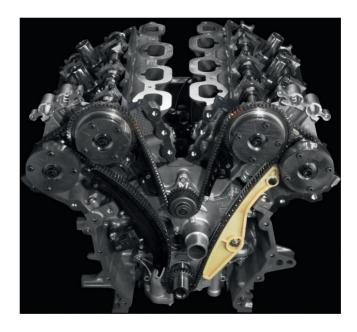
Figure 6.3 V-6 Mustang engine. (Source: Ford Media)
