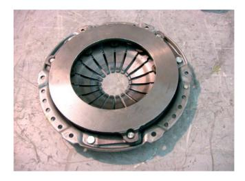
Figure 5.14 Pressure plate
