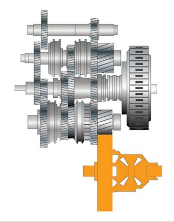
Figure 5.77 Final drive and differential
