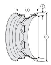
Figure 4.142 Rim sizes: 1, outside and inside rim; 2, flange height; 3, outside and nominal rim diameter
