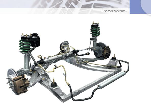
Figure 4.25 Modern front suspension system. (Source: Jaguar/Ford Media)
