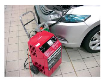
Figure 2.344 Hybrid cars still use a normal 12V battery
