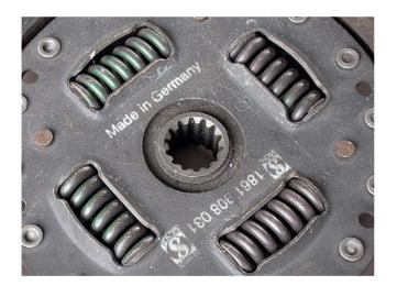
Figure 5.13 Damping springs
