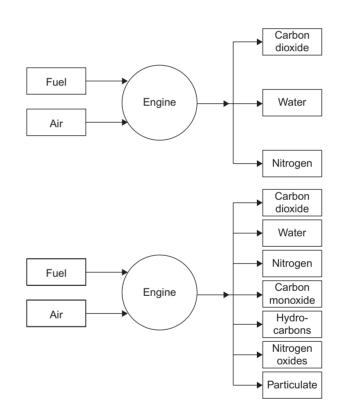
Figure 2.223 Ideal (upper) and incomplete (lower) combustion
