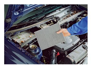
Figure 2.173 Heater intake with pollen filter
