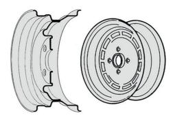
Figure 4.131 Standard wheel design
