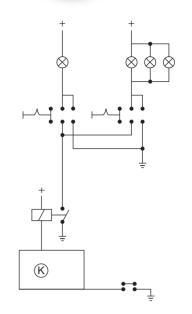
Figure 3.93 Circuit for interior lights
