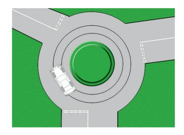
Figure 5.114 The outer wheels travel a greater distance
