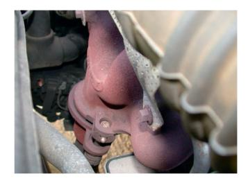
Figure 2.197 Flange connections
