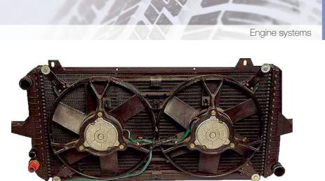
Figure 2.151 Twin electric fans
