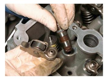
Figure 2.103 Hydraulic lifters
