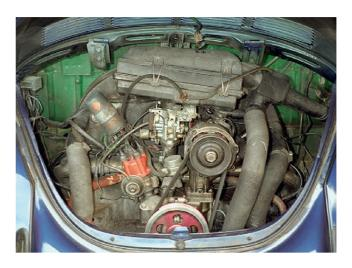
Figure 2.137 Air-cooled system
