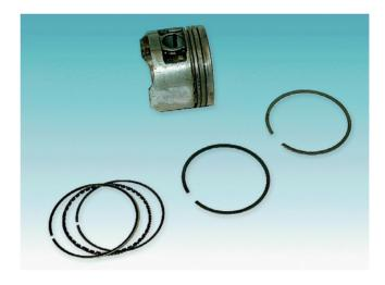
Figure 2.65 Compression and oil control rings
