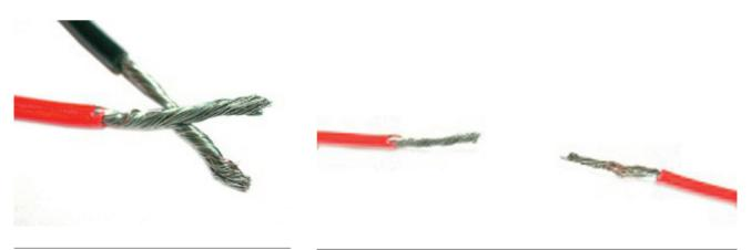
Figure 3.27 Short-circuit
