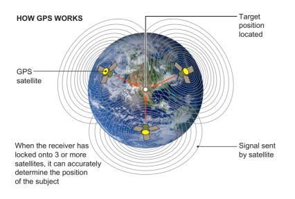
Figure 3.156 How GPS works
