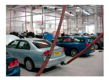
Figure 1.37 Exhaust extraction is an easy precaution to take
