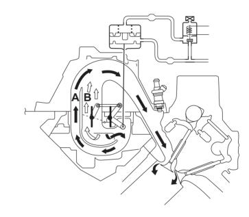
Figure 2.193 Inlet tracts change at different speeds: A: long tract, B: short tract
