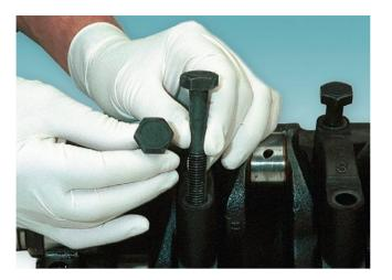
Figure 2.57 Main bearing bolts
