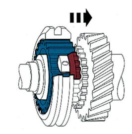
Figure 5.37 Synchronizer synchronizing
