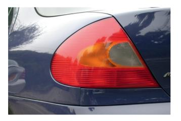
Figure 3.88 Stop and reverse lights form part of the rear light cluster
