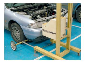
Figure 3.87 Beam setter in use
