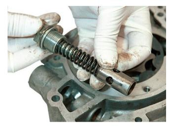
Figure 2.119 Plunger and spring
