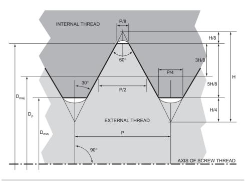
Figure 1.91 ISO metric thread profile
