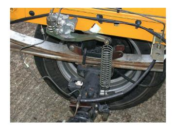
Figure 4.7 Commercial vehicle leaf spring
