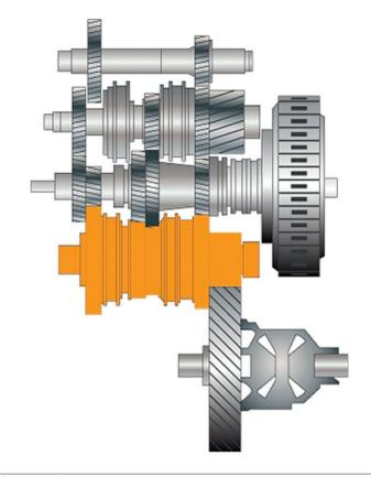
Figure 5.74 Output shaft 1
