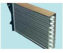
Figure 2.172 Heater radiator
