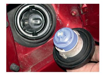
Figure 2.208 Fuel tank cap
