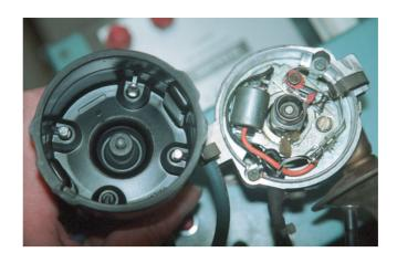
Figure 2.317 Contact breaker system
