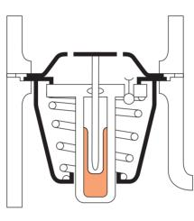
Figure 2.152 Thermostat closed
