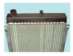
Figure 2.161 Aluminium and plastic radiator
