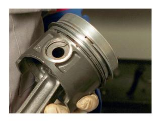
Figure 2.67 Piston pin (gudgeon pin)
