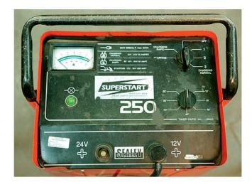
Figure 3.52 Fast charger with time clock
