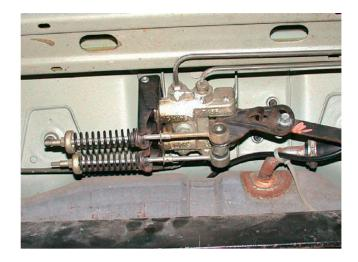
Figure 4.115 Load apportioning valve
