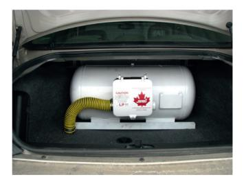
Figure 2.310 Propane tank. (Source: http://www.rasoenterprises.com)
