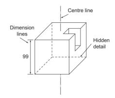
Figure 1.65 A three-dimensional (3D) representation (oblique projection)
