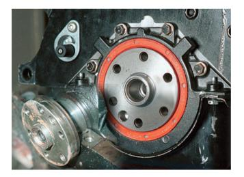
Figure 2.77 Radial lip oil seal
