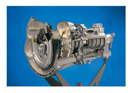
Figure 5.22 Lincoln five-speed rear-wheel drive gearbox. (Source: Ford Media)
