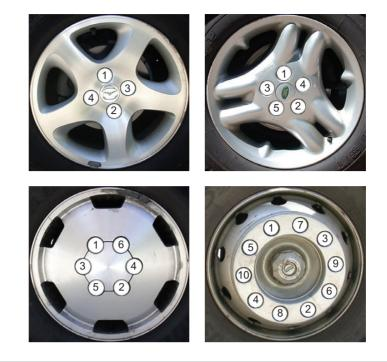
Figure 4.141 Torque sequences
