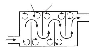
Figure 2.195 Baffle silencer
