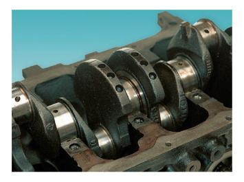
Figure 2.76 Journals in position in the engine block
