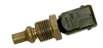
Figure 3.141 Temperature sensor
