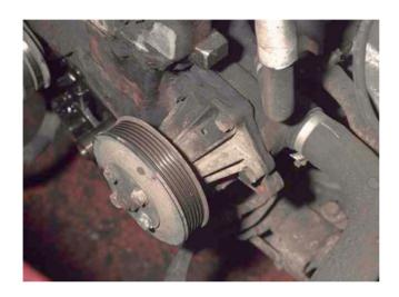
Figure 2.164 External water pump
